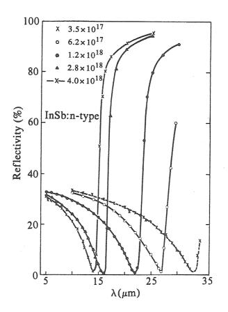
The above graph shows the reflectivity *R* versus wavelength  $\lambda$  for an extrinsically-doped semiconductor, InSb, which has a semiconductor band gap of around 0.2 eV, with different free-carrier concentrations as indicated (in units of cm<sup>-3</sup>).
